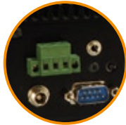
ECW-281B has two power input interfaces: 3-pin terminal block or DC power jack.
